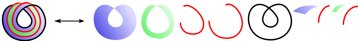
Figure 6.1: Left: Example of figure that was challenging to author with current tools. Right: Exploded view of the figure revealing the 9 independent Bézier curves that had to be created in order to achieve the desired outcome. Not only determining how to achieve the desired depth-ordering was a puzzle on its own, but even once solved, any edit of the figure was made painfully complicated due to all pieces having to be edited independently, and carefully aligned to prevent any visible seam.
