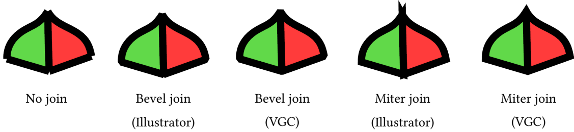
Figure 4.24: Illustrator (except when using LivePaint) cannot represent multiway joins, thus fails to render them correctly: incident faces are rendered independently. With the VGC, we are aware of multiway joins and hence can improve the rendering, as illustrated here with the two common styles “bevel” and “miter”.
